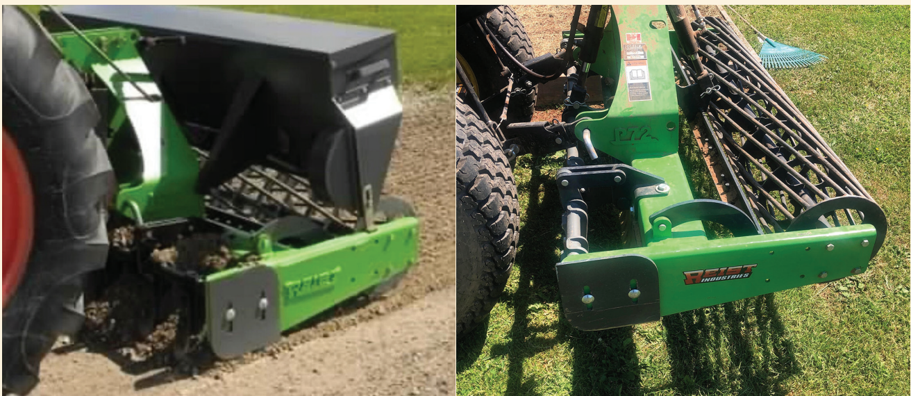
A compact seeder well suited for seedling soil conservation structures. The rolling basket helps reduce rills.
